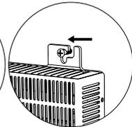
6. Align the peg with the notch and hold the product. The mounting ear is installed.
