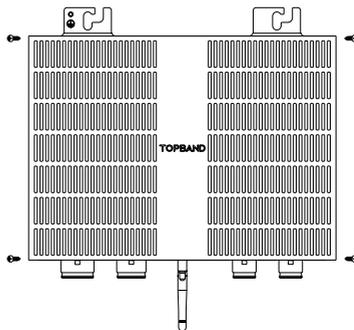
1. Align the four Angle mounting holes of the product with the four positioning holes of the wall.
